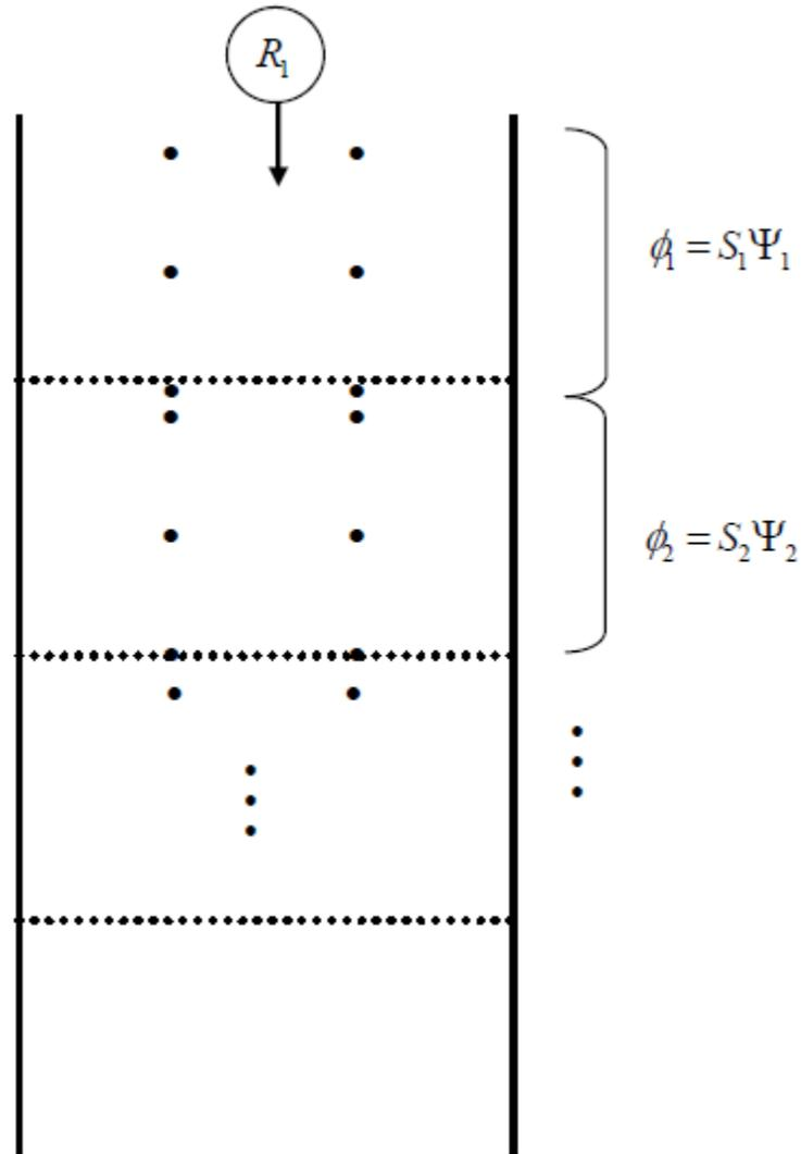
**Figure 4.2.** Schematic of a Release ( $R_1$ ) of Acoustic-tagged Juvenile Salmonids with Downriver Arrays to Estimate Perceived Survivals ( $\phi_i$ ). Inter-reach nodes ( $\bullet$ ) are used to estimate abundance of live, tagged juveniles in the reaches over time to differentiate survival and residualization processes.
