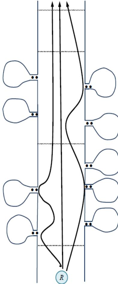
**Figure 4.4.** Schematic of an Acoustic-Tag, Release-Recapture Design to Estimate Juvenile Salmonid Survival, Site Use Patterns, and Near-Term Benefits of Site Use. Cross-river arrays (dotted line) and individual hydrophones (•) at estuary openings are delineated. Three possible fish tracks are illustrated.
